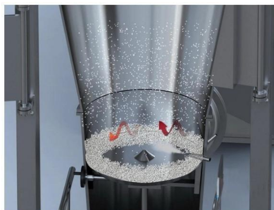
Figure: 5 SUB COATING (FBC)
