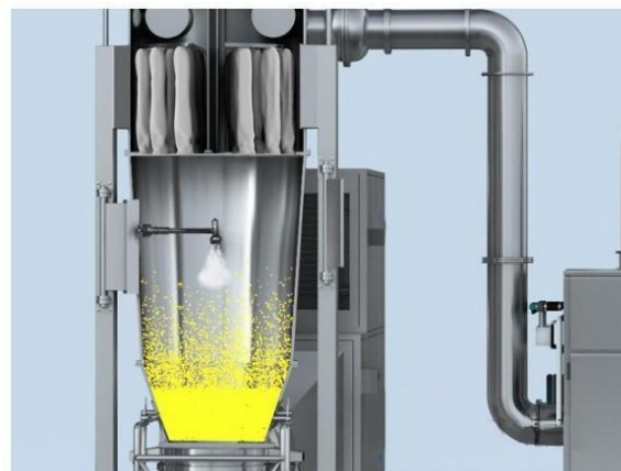
Figure: 4 fluid bed granulator with a top spray system
