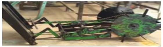
ground. When the seedlings are removed from their trays, the fork attached to the shaft supports them horizontally on the skid. A chain and sprocket system is used to move the wheel and shaft by hand..
