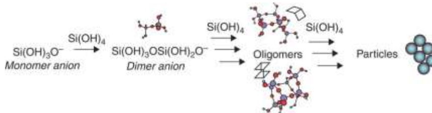
FIG. 1. The polymerization of monomeric silicic acid to form larger silica particles proceeds through various condensation reactions with dimers, oligomers and aggregates as intermediates.
