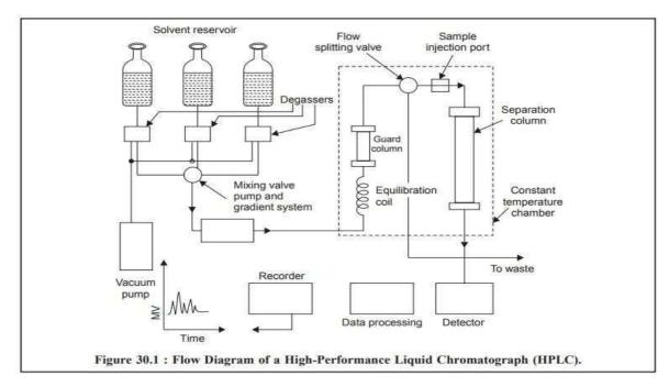
This schematic diagram shows the basic instrument for HPLC [51]
